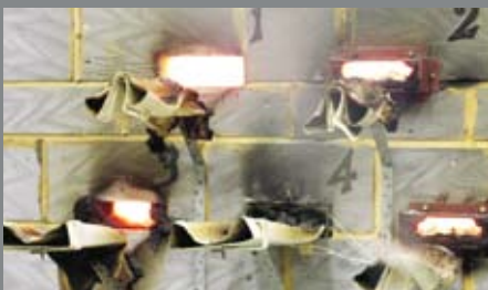
After 2 hours: FireBrake (No. 4) has maintained its fire stop closure whilst the traditional products failed.
