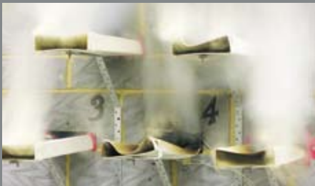
After 5 minutes: The Domus FireBrake (No. 4) is already creating an effective fire stop seal.
